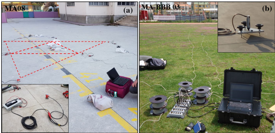
Fig. 2 Array plan and two different microtremor sets: a ITU-TITECH MA measurements and b Bursa Metropolitan Municipality MA-BBB measurements
