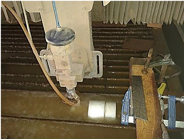
Fig. 3. Submerged abrasive water jet experimental setup.
