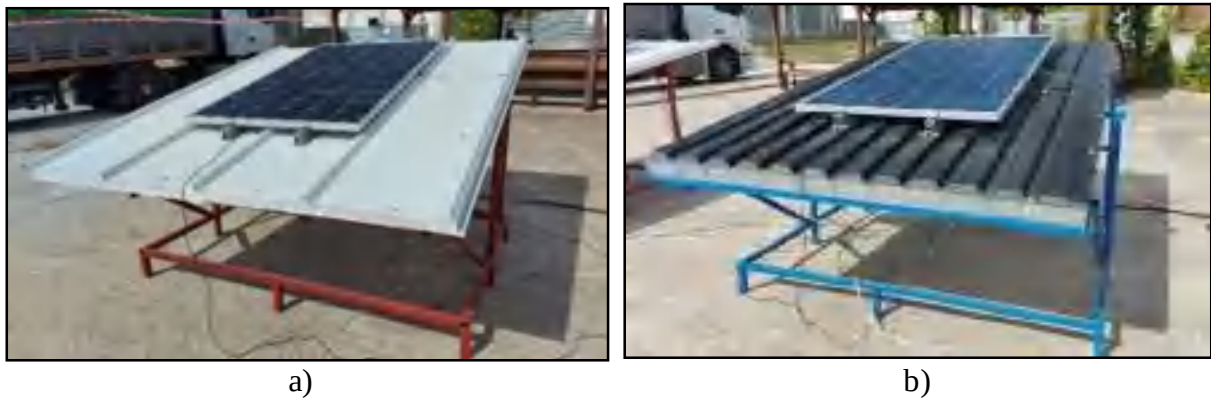
Figure 4. a) PV and b) PV/T systems
