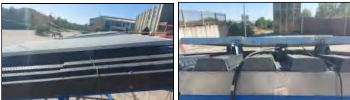
Figure 10. Temperature sensors installed on the PV/T system
