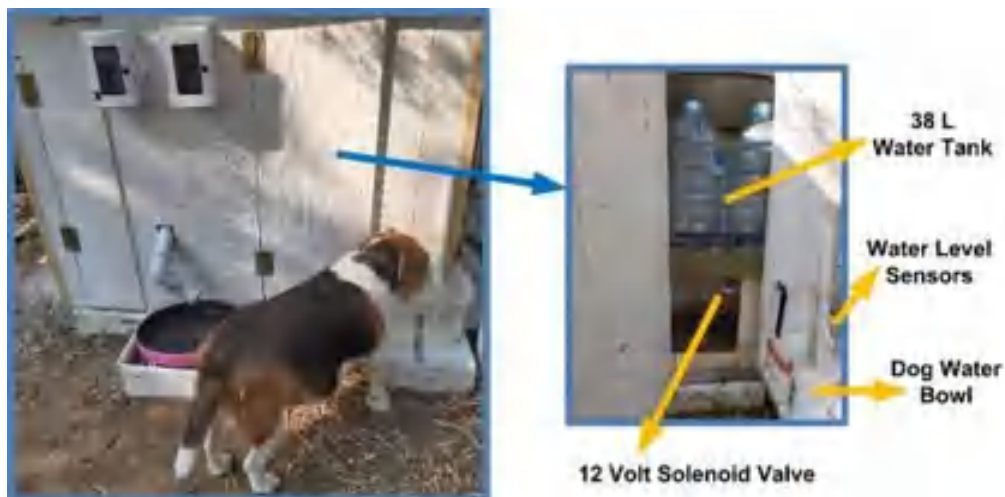
Figure 12. Photograph of the parts of the proposed system related to water
