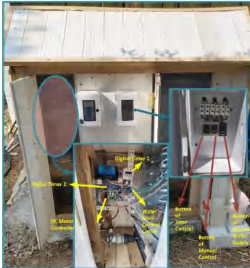
Figure 13. Control unit of the automatic pet feeder and water dispenser
