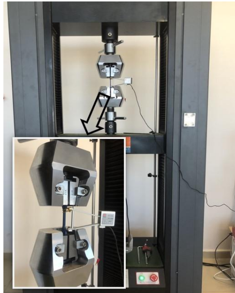
Fig. 1. Overview of the tensile test machine (KAEU-Mechanical Engineering Mechanics Lab.).
