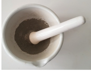
FotoĖraf 10. Porselen havan ile d v lerek toz haline getirilen sediment  rne leri. Photo 10. Samples of sediment pulverized with porcelain mortar.
