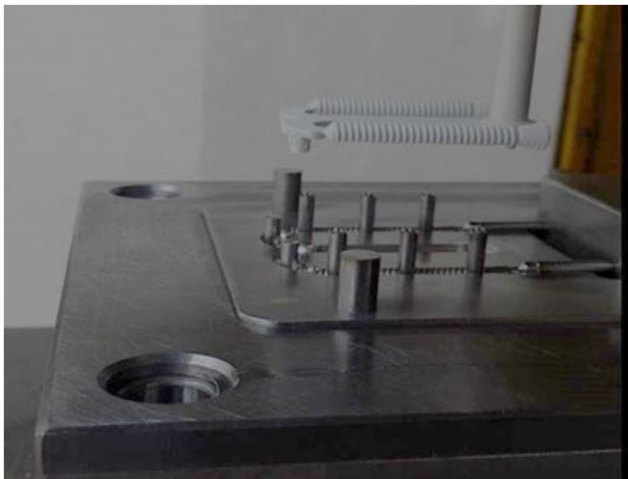
Fig. 5 – Green part production with 60% feedstock by volume.
