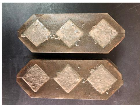
Fig. 5. Specimens used for the compressive strength experiment.
